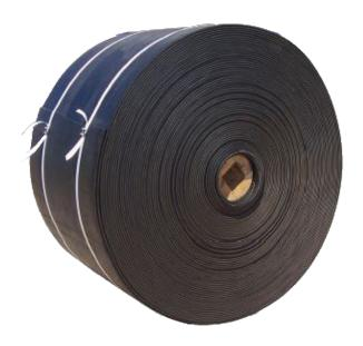
▶ **TekTip:** When storing a belt for long periods the roll should be placed on to an A-frame and periodically turned in order that the inner pressure does not continuously affect the same area.
