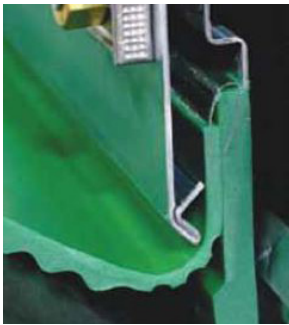
Low friction PU skirting with quick release clamp system
